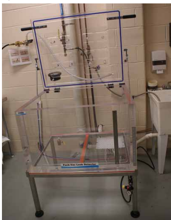
Figure 1. Haug Pac-Vac Leak Detector
