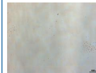
Image 3: Vendor B - Composite Image of Container "as received" from another lot produced differently from Vendor A. Container showed a smoother surface appearance upon comparison to Vendor A's containers.
