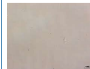
Image 6: Vendor B - Composite Image of Container from another lot produced differently from the "suspect" lot after being challenged. Container showed a smooth surface appearance with little or no change.
