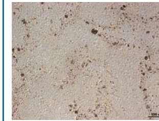
Image 1: Vendor A - Composite Image of Container "as received" from "suspect" lot. In the case of the "suspect" container, this showed an interlocking lattice network of small defects, suggestive of cracks, outlining areas suggestive of flakes.
