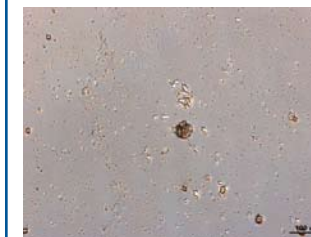
Image 2: Vendor A - Composite Image of Container "as received" from another lot produced similarly to the "suspect" lot. In the case of another lot produced similarly to the "suspect" container, this showed an interlocking lattice network of small defects, suggestive of cracks, outlining areas suggestive of flakes.
