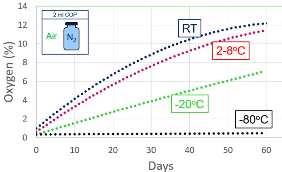
Figure 3. Oxygen Concentration vs Time and Temperature for 2 mL Daikyo Crystal Zenith<sup>®</sup> COP Vial Primary Package Systems. Elastomer stoppers were NovaPure<sup>®</sup> 1358 / 4023/50 Gray (i.e., with FluroTec<sup>®</sup> barrier film). Measurement was by frequency modulated spectroscopy headspace analysis. (14)
