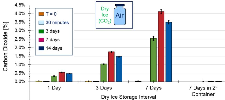
Figure 5. Carbon Dioxide Concentration vs Time for 5 mL Daikyo Crystal Zenith<sup>®</sup> COP Vial Containment Systems after Storage in Dry Ice (-78°C) and Storage in Air (room temperature). Elastomer stoppers were 20mm NovaPure<sup>®</sup> 1343 / 4023/50 Gray (i.e., with FluroTec<sup>®</sup> barrier film). Measurement was by frequency modulated spectroscopy headspace analysis. (14)
