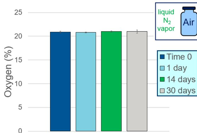
Figure 4. Oxygen Concentration vs Time for 2 mL Daikyo Crystal Zenith<sup>®</sup> COP Vial Primary Package Systems at -180°C. Elastomer stoppers were NovaPure<sup>®</sup> 1358 / 4023/50 Gray (i.e., with FluroTec<sup>®</sup> barrier film). Measurement was by frequency modulated spectroscopy headspace analysis.
